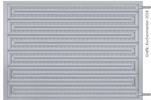
Abb. 3: Thermoölführender Radiator (Schema)
